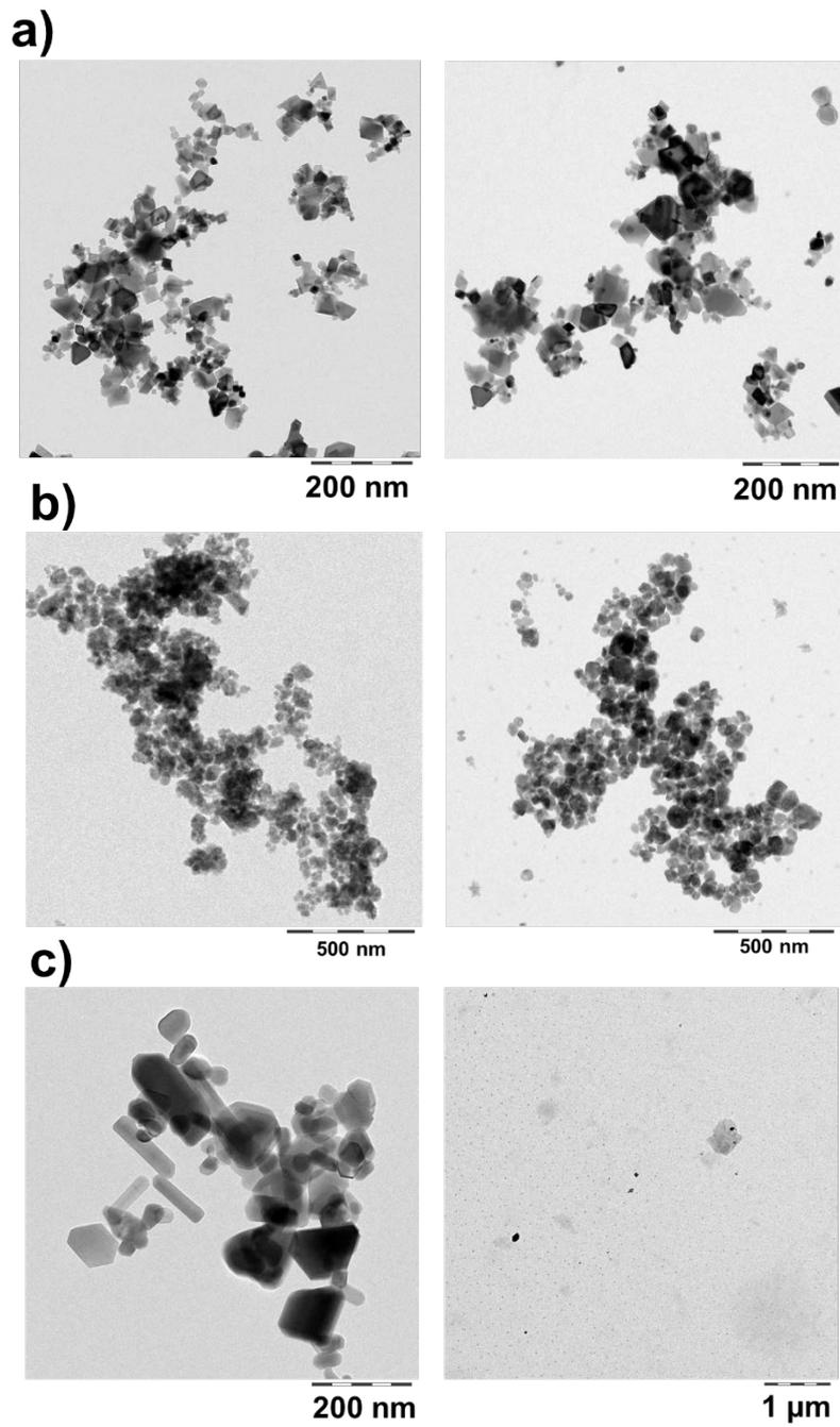
Figure 10.3: TEM images of a) CeO<sub>2</sub> NM212, b) BaSO<sub>4</sub> NM220 and c) ZnO NM110 (reproduced from Koltermann-Jüilly et al. 2018). Left: before dissolution testing. Right: after 75h dissolution testing in pH4.5 PSF lysosomal simulant.
