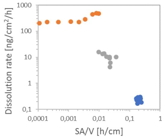
Figure 10.2: Example of a quality control by measuring dissolution rates across a range of different materials BaSO<sub>4</sub> NM220 1,05 mg (gray), CuO 1.56 mg (orange), SiO<sub>2</sub> NM203 0,144 mg (blue) and plotting them against SA/V.
