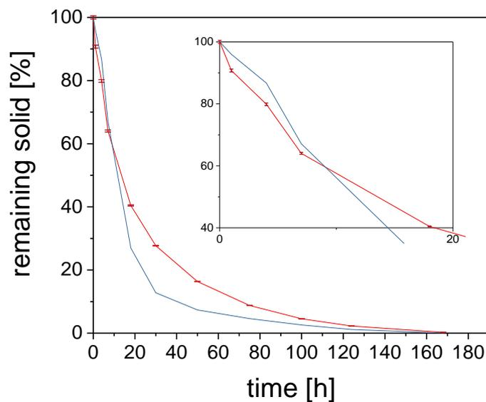
Figure 10.1: Dissolution kinetics of ZnO NM110 (red) and ZnO NM111 (blue) (reproduced from Koltermann-Jülly et al. 2018).
