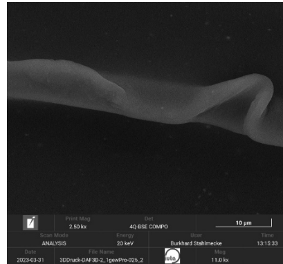
Annex 17: Exemplary images of the SEM-analysis of DAF3D-2 1 wt% printed samples taken at a magnification of 1.1 kx (left) and 11 kx (right).
