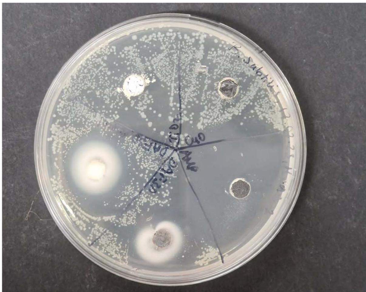
Figure 17: Zone of inhibition for B. Subtilis for (clockwise) Ampicillin, DAF3D-1 and DAF3D-2, TiO 2 and CuO.
