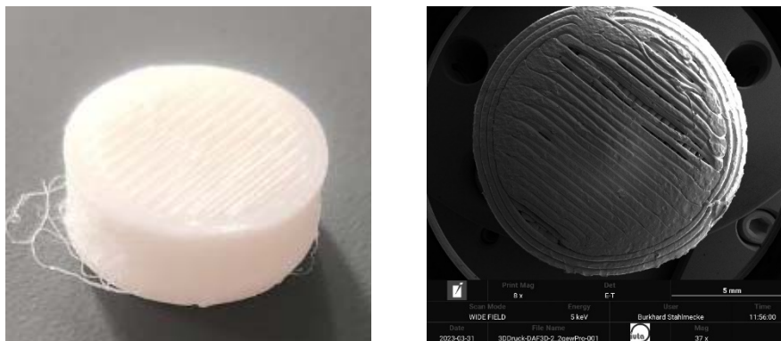
Figure 28: Printed sample of PA12 used for SEM-analysis.
