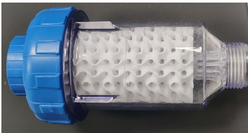
Figure 35: Printed gyroid filter bed encased in filter housing. Made from pure PA12. Printed in two parts for a total dimension of 70 x 42 mm.
