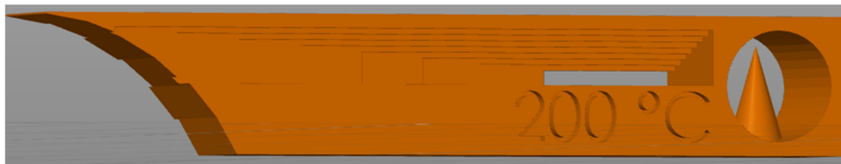
Figure 21: Unit of a Temptower. 10 x 10 x 100 mm 3 . Several characteristics typical for 3D-prints can be observed. Stringing at the cone on the right side. Bridges in the middle and overhangs at the left structure.
