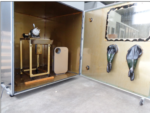
3 m³ chamber for aging with cigarette smoke
