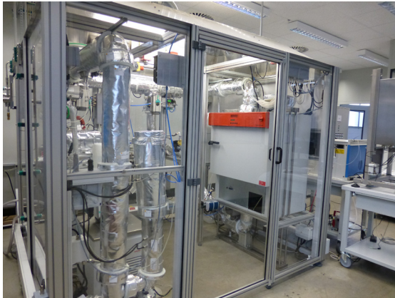
Test rig for toxic and nontoxic gases
