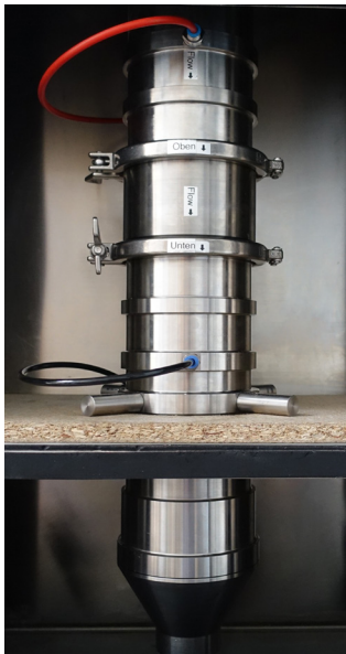
Test adsorber (ISO 10121-1)
